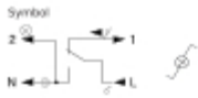
Two-way switch with indicator light as one-way switch with indicator light or heating emergency switch
