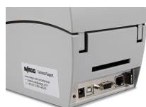
Secure Bluetooth® (item number 258-5102) or WiFi Dongle (item number 258-5103) in the USB-A interface.
