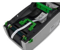
Guide the marker strip over the roller.
