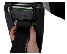
Insert the entire core of the ink ribbon at the bottom.
