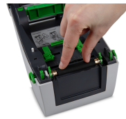
Secure the appropriate roller in the printer.
